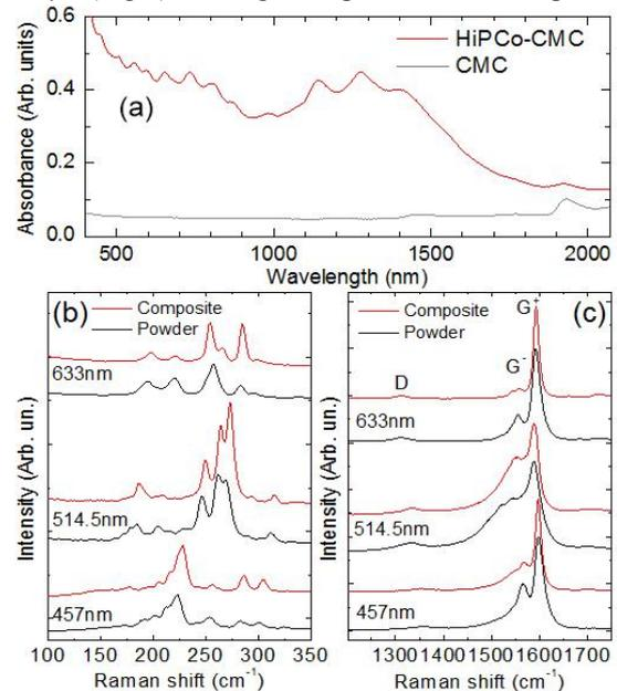
Fig.2(a) Absorbance of HiPCo SWNT and CMC. Raman spectra of HiPCo SWNT at 457,514,633nm for powders (black lines) and dispersions (red lines) in the (b) RBM and (c) G peak region.
