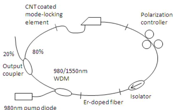
Fig. 3 Schematic of the mode-locked laser.
