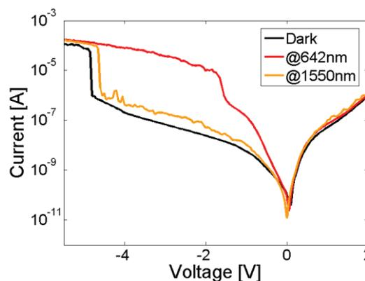
Fig 2. I-V characteristics under illumination
