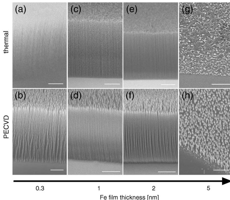
Fig. 4. SEM images of CNTs grown from 0.3-, 1-, 2- and 5-nm-thick Fe films under purely thermal and DC PECVD conditions. Growth conditions were:  $\sim 550$  °C and 1:4  $\text{C}_2\text{H}_2/\text{NH}_3$  gas mixture. For DC PECVD-grown CNTs, a 600 V DC bias was applied. Scale bars are: 2  $\mu\text{m}$  (a, b, g), 5  $\mu\text{m}$  (c–f), 1  $\mu\text{m}$  (h).
