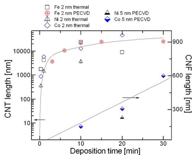
Fig. 6. (Color online) Growth saturation plot of CNTs grown under purely thermal and DC PECVD from 2-nm-thick catalyst films, compared with CNFs grown from thicker (5 nm) catalyst films under DC PECVD conditions. Growth temperatures are  $\sim 550^\circ C$  for CNTs (left axis) and  $\sim 450^\circ C$  for CNFs (right axis).
