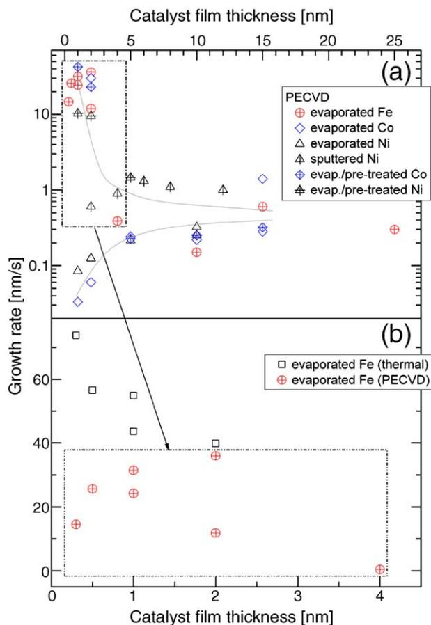
Fig. 7. (Color online) Variation of average CNT/CNF growth rate as a function of catalyst thin film thickness for Fe, Co and Ni-catalyzed CNT/CNF samples grown in DC PECVD conditions (a), and comparison between CNTs grown from Fe only, in purely thermal and DC PECVD conditions (b).
