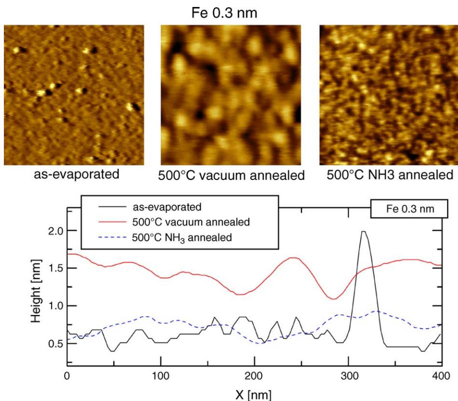
Fig. 2. (Color online) AFM analysis of 0.3-nm-thick Fe film subject to different pre-treatment stages: as-evaporated, annealed in vacuum ( $<10^{-5}$  mbar pressure) at  $\sim 500$  °C and annealed in  $\text{NH}_3$  (0.6 mbar pressure) at  $\sim 500$  °C. The section analysis shows the topography profile along sample lines in the respective amplitude image. Image scan dimensions are  $400 \times 400 \text{ nm}^2$ .
