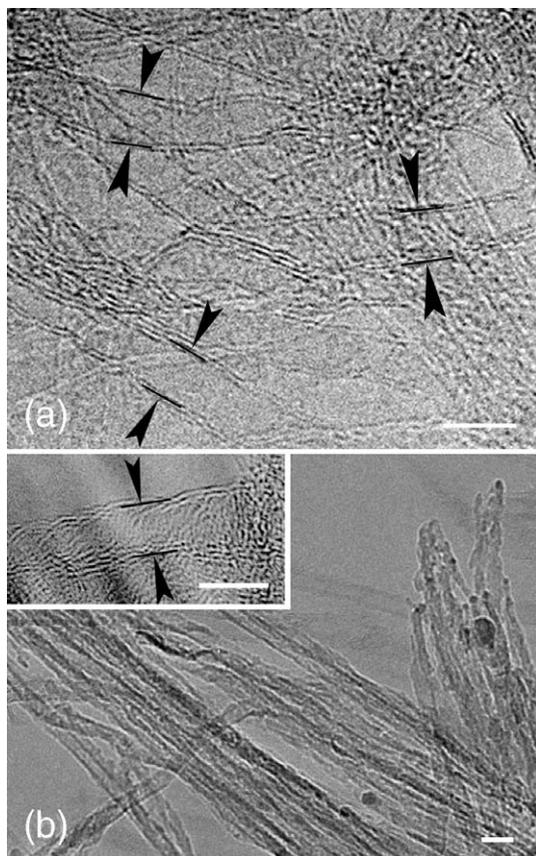
Fig. 5. HRTEM analysis of thermally (a) and DC PECVD-grown (b) CNTs catalyzed from 2-nm-thick Fe films. Scale bars are: 5 nm (a), 20 nm (b), 5 nm (inset).
