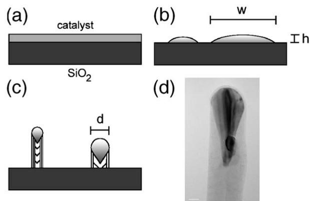
Fig. 3. Schematic of the CNT/CNF growth mechanism. The initial thin catalyst film (a) is heated up to the desired temperature and splits up into islands (b). Nanotubes grow as the hydrocarbon precursor is fed into the chamber (c), and a HRTEM image shows an example of CNF grown with tip-growth mechanism (d, scale bar: 20 nm).
