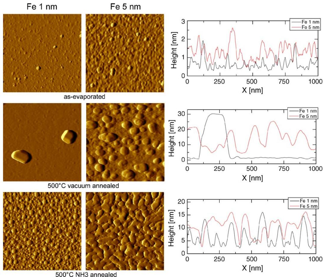
Fig. 1. (Color online) AFM analysis of 1- and 5-nm-thick Fe films subject to different pre-treatment stages: as-evaporated, annealed in vacuum ( $<10^{-5}$  mbar pressure) at  $\sim 500$   $^\circ\text{C}$  and annealed in  $\text{NH}_3$  (0.6 mbar pressure) at  $\sim 500$   $^\circ\text{C}$ . The section analysis show the topography profile along sample lines in the respective amplitude image. Image scan dimensions are  $1 \times 1 \mu\text{m}^2$ .
