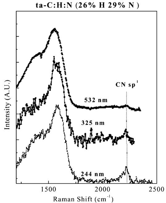
Fig. 5. MW Raman spectra for hydrogenated CN films. Note that again CN–sp<sup>1</sup> bonds are clearly detected at UV–excitation.
