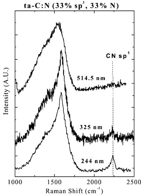
Fig. 4. Raman spectra of a ta-C:N sample measured at different excitation wavelengths. Notice how the 'shape' of the spectra changes with the laser wavelength. CN–sp<sup>1</sup> bonds are remarkably enhanced for UV–Raman.
