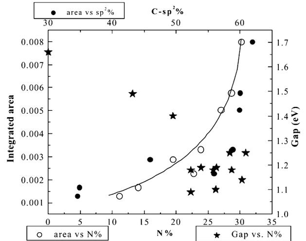
Fig. 9. Tauc optical gaps (right: y-axis) and IR integrated area from  $900$  to  $1800\text{ cm}^{-1}$  vs. nitrogen content (bottom: x-axis) and vs. CC– $sp^2\%$  (top: x-axis). Corresponding to the series of hydrogenated samples deposited by a mixture of  $C_2H_2/N_2$ . The line is only a guide for the eyes.
