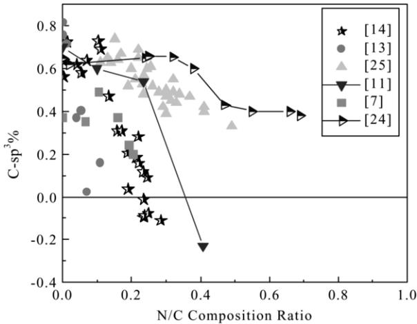
Fig. 7. Variation of the C–C  $sp^3$  fraction as measured by EELS. Negative values in the  $sp^3$  fraction are indicative of a significant fraction of  $sp^1$  bonds. These are usually neglected in the standard C– $sp^3$  calculations because carbon films hardly content any CC– $sp^1$  bonds. However, IR and Raman spectra of CN films clearly show the presence of CN– $sp^1$  bonds.
