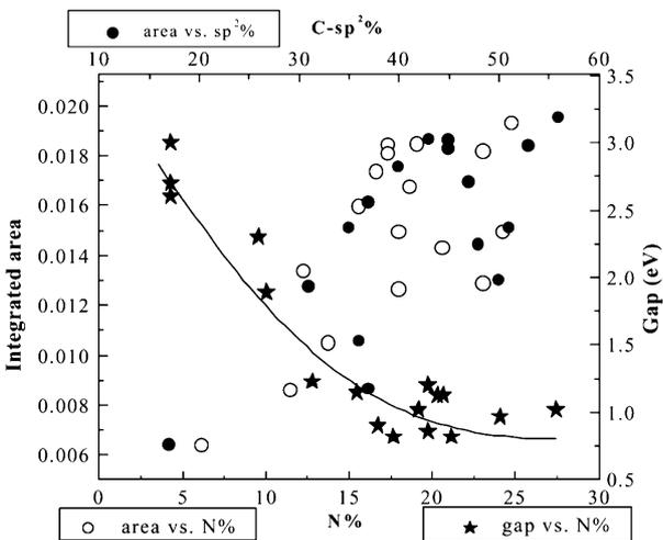
Fig. 8. Tauc optical gaps (right: y-axis) and IR integrated area from  $900$  to  $1800\text{ cm}^{-1}$  vs. nitrogen content (bottom: x-axis) and vs. CC– $sp^2\%$  (top: x-axis). Corresponding to a series of ta-C:N samples. The line is only a guide for the eyes.
