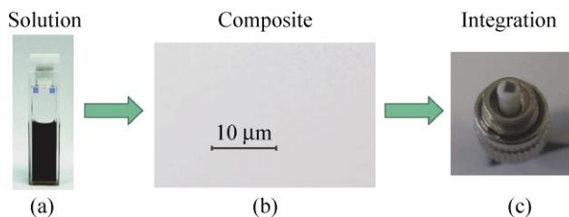
**Figure 2** Preparation and integration of the SWNT-PVA composite: (a) photograph of the SWNT dispersion after ultrasonication; (b) optical micrograph of the SWNT-PVA composite showing no aggregation; (c) integration of ~2  $\text{mm}^2$  of the composite to a fiber connector
