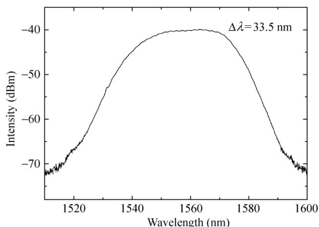
**Figure 6** Typical output spectrum, with bandwidth  $\sim 33.5$  nm
