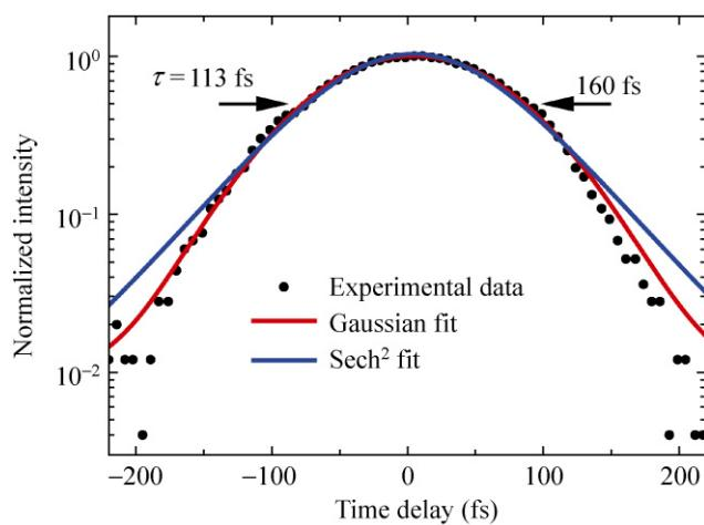
**Figure 7** Autocorrelation trace, with Gaussian and  $\text{sech}^2$  fits
