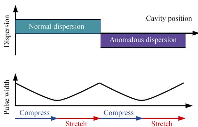
**Figure 1** Simplified scheme of a stretched-pulse laser, with the dispersion map (top) and pulse width distribution (bottom). Normal (positive) and anomalous (negative) dispersion are marked with different colours
