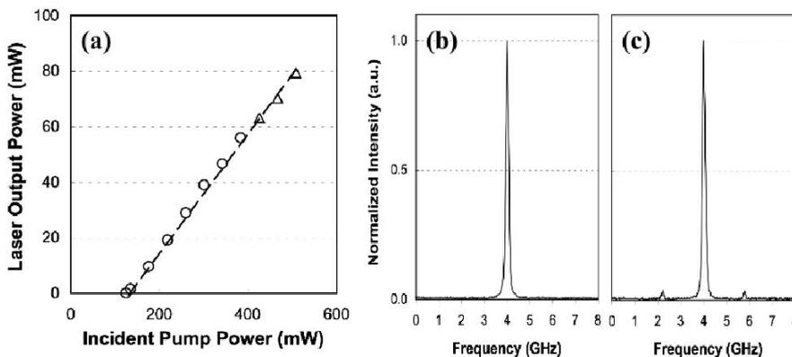
Figure 2. (a) Input-output characteristic of the 5.5-cm long waveguide laser cavity: single mode operation (circles); slightly multimodal regime (triangles). Fabry Perot spectrum (a) in SM operation at 55 mW output power and (c) in slightly multimodal regime at 80 mW output power.
