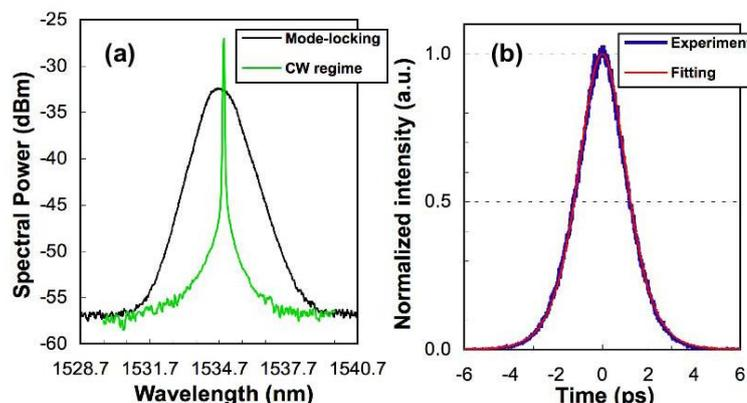
Figure 4. (a) Laser output spectrum in continuous wave and mode-locking regimes. (b) Autocorrelation trace of the mode-locking pulse.
