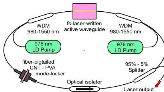
Figure 3. Schematic set up of the mode-locked ring laser cavity configuration.
