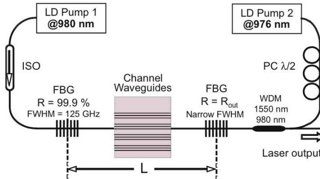
Figure 1. Waveguide linear laser cavity. A bi-directional pumping scheme is adopted. Pump interaction is removed by means of an optical isolator (ISO) and a half-wave polarization controller (PC  $\lambda/2$ ).
