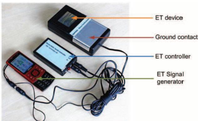
FIG. 2 Graphene ET system. Upon receiving electrical signal from the generator, the controller sends stimulating signals to the visually transparent ET device. The user completes the electrical circuit by touching the ground contact.
