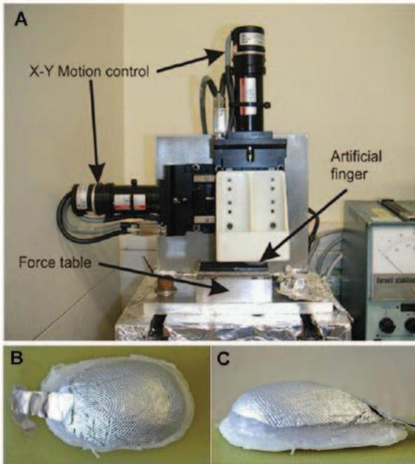
FIG. 4: a) Setup for the dynamic friction test measurement during ET device operation. The ET device is secured on a backing layer. Photograph of the B) top and C) side view of the artificial finger.
