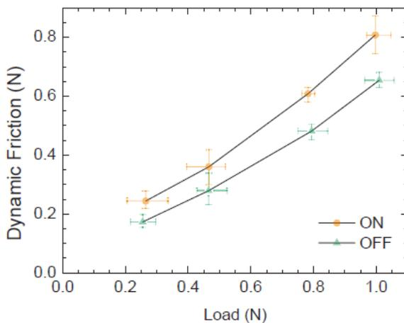
FIG. 5: Change in dynamic friction between the artificial finger and ET device touch surface against different loads in ON and OFF states.
