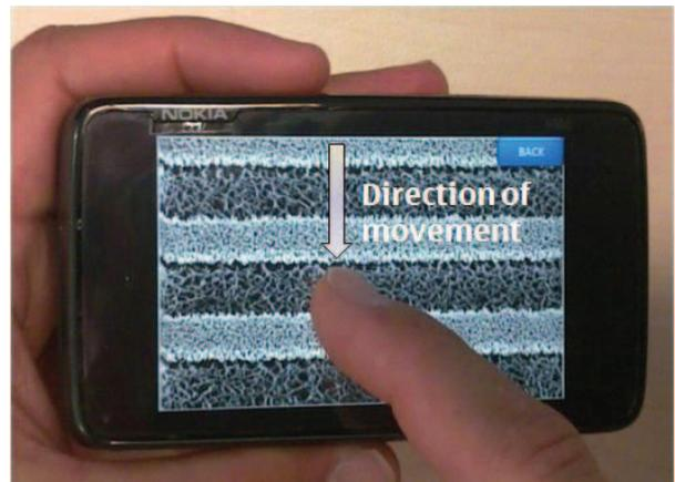
FIG 3 Implementation of the ET system in accordance with actual touch coordinates on the display. Different tactile signals are generated on the alternating stripes.
